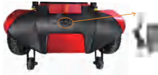
Then open the rear charging socket and insert the plug
