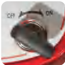
Close the ship stype switch or key switch
